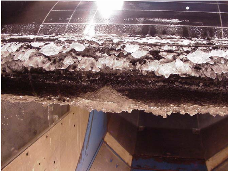
Figure 3. Hybrid NACA 23012 2D (simulating a 72-inch chord airfoil) model intercycle ice before the third cycle of a pneumatic deicing boot. Three-minute boot cycle intervals were used. The test was performed in 14 CFR part 25, Appendix C Maximum Continuous Icing Conditions. (Static temperature = 14°F, LWC = 0.45 g/m 3 , MVD = 20 micrometers, Spray time = 6:11 min., Tunnel airflow speed = 195 mph, Model AOA = 4°.)
